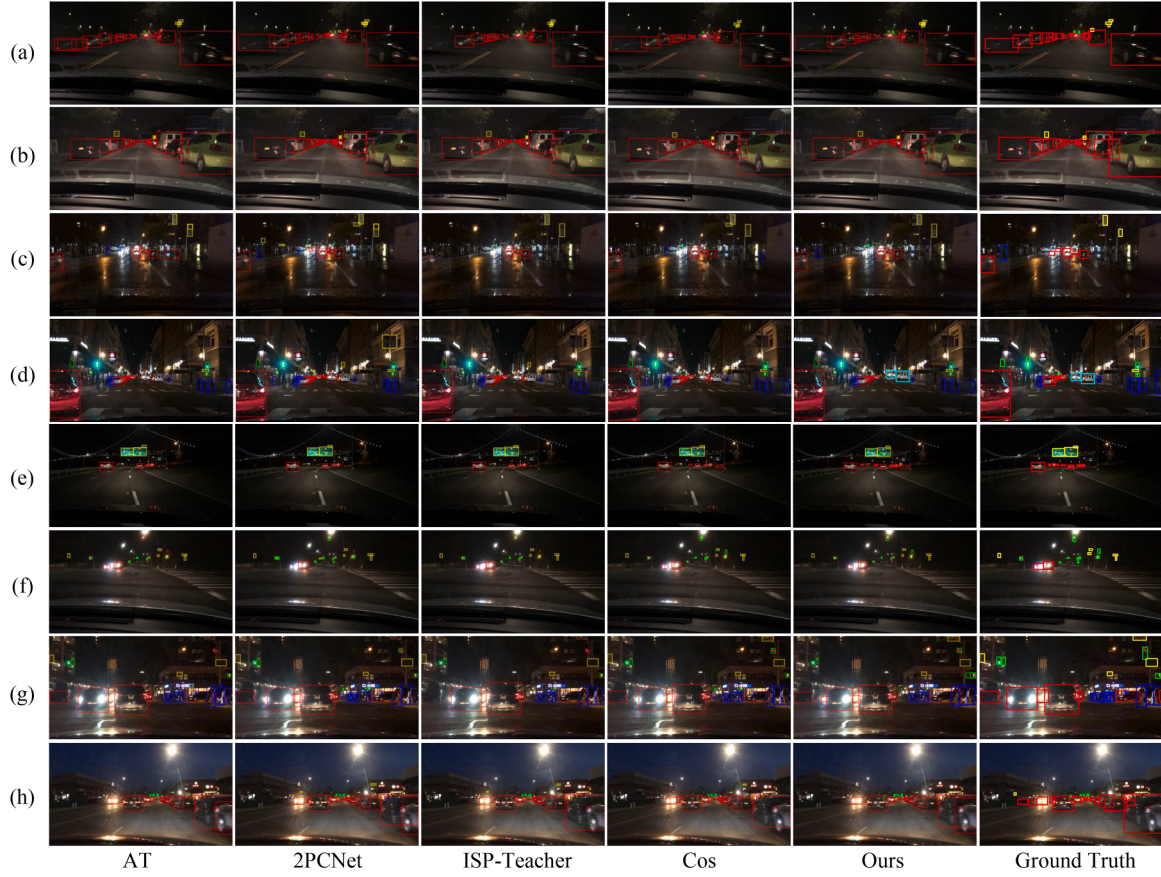
Fig. 8. Examples of detection results on BDD100k dataset. For each row of figure, (a) and (b) are dark scenes in clear weather, (c) is the dark scene in rainy weather, (d) contains minority class ‘Bus’, (e) and (f) are small instances of different classes. We also show some failed examples of our method in (g) and (h). Different colored boxes denote different classes, i.e. red box denotes ‘Car’, blue box denotes ‘Pedestrian’, cyan box denotes ‘Bus’, yellow box denotes ‘Traffic Sign’ and green box denotes ‘Traffic Light’. (For interpretation of the references to colour in this figure legend, the reader is referred to the web version of this article.)
